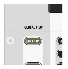
If the second layer option is activated, Vista 8 may display the label and real time metering of both layers at the same time. In order to activate this label view, press LABEL TYPE several times until the label display area on the Vistonics<sup>®</sup> screen shows the labels of both layers. This label of the second layer appears only if there is a channel assigned to that strip on both layers. Use the Strip Setup dialog on the graphic controller screen to do this.
