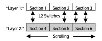
It is still possible to globally switch to the second layer by pressing the section navigator keys 4...6. This will activate the L2 keys on each strip of the console surface, indicating that the operator is now looking at the lower half of the console.
