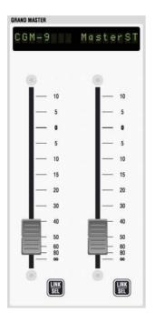
Vista 8's control bay also hosts two "grand master" faders. The user determines which two faders are most important for him and to which he wants constant access. This may be very useful as an "emergency access" to very important output faders, since these faders will never scroll or be switched over in any way. Which two channels are controlled by these faders is defined in the top right corner of page 2 (Control Bay tab) of the strip setup window, as shown below.
