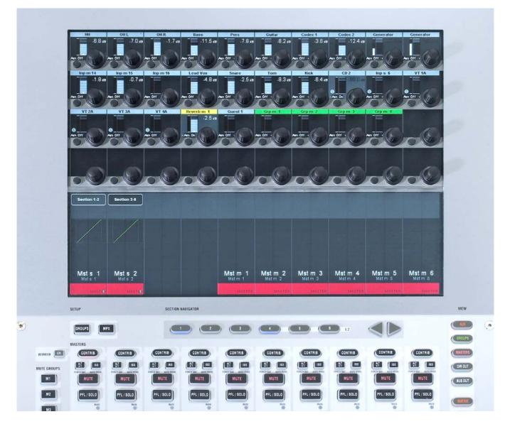
It is extremely easy to adjust a balance of e.g. a matrix output without accessing the fader strips of the contributing channels.
